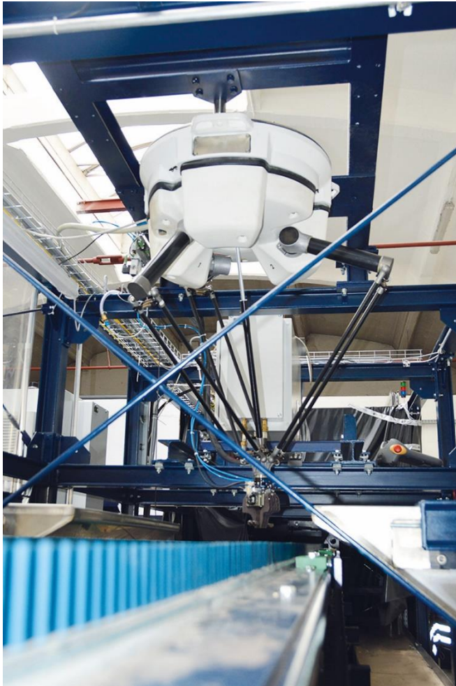
Image 3: The pilot plant for laser-based recycling, which was created in the PLUS project, is suitable for the automatic processing of high-speed steels (HSS), for example. © Cronimet Ferroleg. GmbH, Karlsruhe, Germany.
