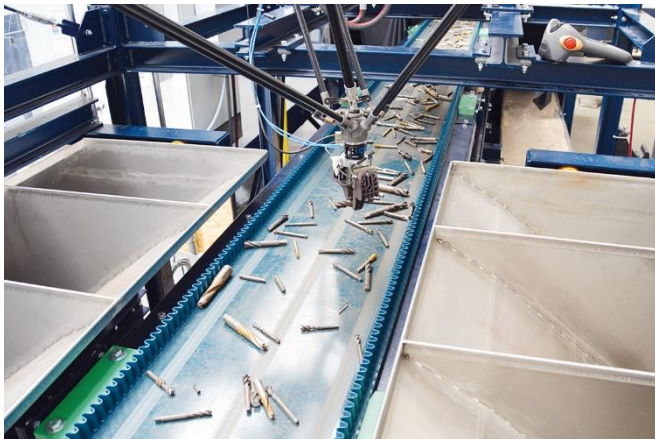
Image 2: With a laser-based sorting process developed in the BMBF PLUS project, valuable alloys can be efficiently recovered from metal scrap. © Cronimet Ferroleq. GmbH, Karlsruhe, Germany.
